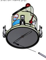
3. Place the upper part down onto the test pot, and snap the quick-release latches downward. Make sure that the markings on the top and bottom parts are in line, and that the angles of the claps are
