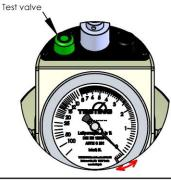
10. Screw down the threaded tube onto the left ball shut-off valve. Let the tube hang into a suitable graduated cylinder and open the ball shut-off valve. Operate the TEST valve and pump with the hand pump until 100ml (1-litre unit), 250ml (5-litre unit), or 400ml (8-litre unit of water has flowed out. Then close the left ball Hand pump
