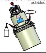
7. While the water is still flowing consistently, slowly shut off the water flow gradually and close the two shut-off valves.
