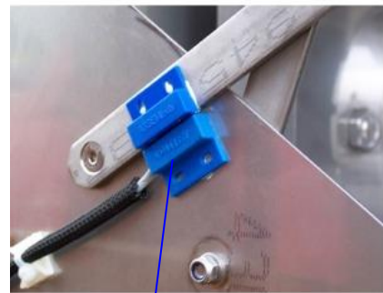
Glass shield safety switch
