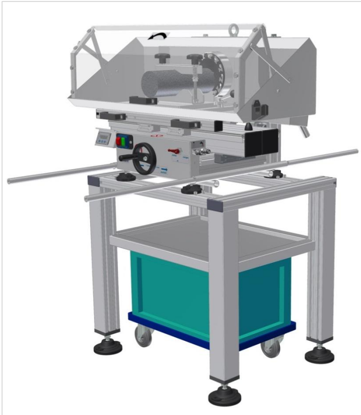
Image above: Grinder sitting on the bottom bed, with supporting frame and grit trap container
